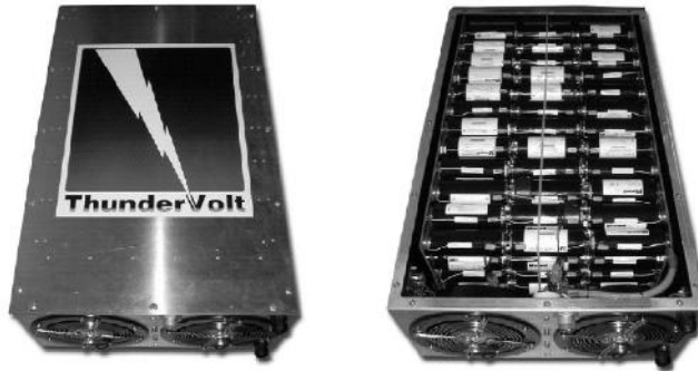
Figure 16. Maxwell's ultra capacitors. a) overview; b) data of a package; c) data of an individual component (European 6F project HYHEELS with the author's collaboration)
